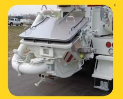
Putzmeister's EZ Clean Out RS 907A hopper is engineered for performance and easy maintenance. Offering 19.4 cu. ft. (550L) capacity, the hopper features hard-faced remixer paddles and vibrator. The unique design of the splash guard protects the unit from splattering during pumping and folds down and latches to cover the hopper during transit.
