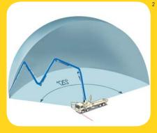
For enhanced job site versatility, Putzmeister's unique OSS system allows the operator to reduce the outrigger extension on one side of the unit to create a smaller overall machine footprint. Utilizing a series of sensors, OSS enables the unit to maintain a defined and safe 120 degree working envelope on space restrictive sites that demand a larger boom.
