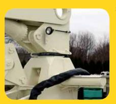
The 38Z-Meter boom features a simple mechanical rack and pinion design for improved weight distribution and easy serviceablility. Putting the pump closer to the cab, rack and pinion slewing offers greater reach than rotation bearings on lighter weight models. Specially designed teeth in the system offer smooth rotation and prevent backlash in the swing gears.
